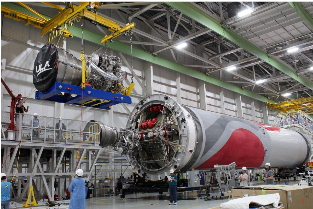
ULA technicians guide a Blue Origin BE-4 engine onto the aft end of a Vulcan booster. Credit: United Launch Alliance
