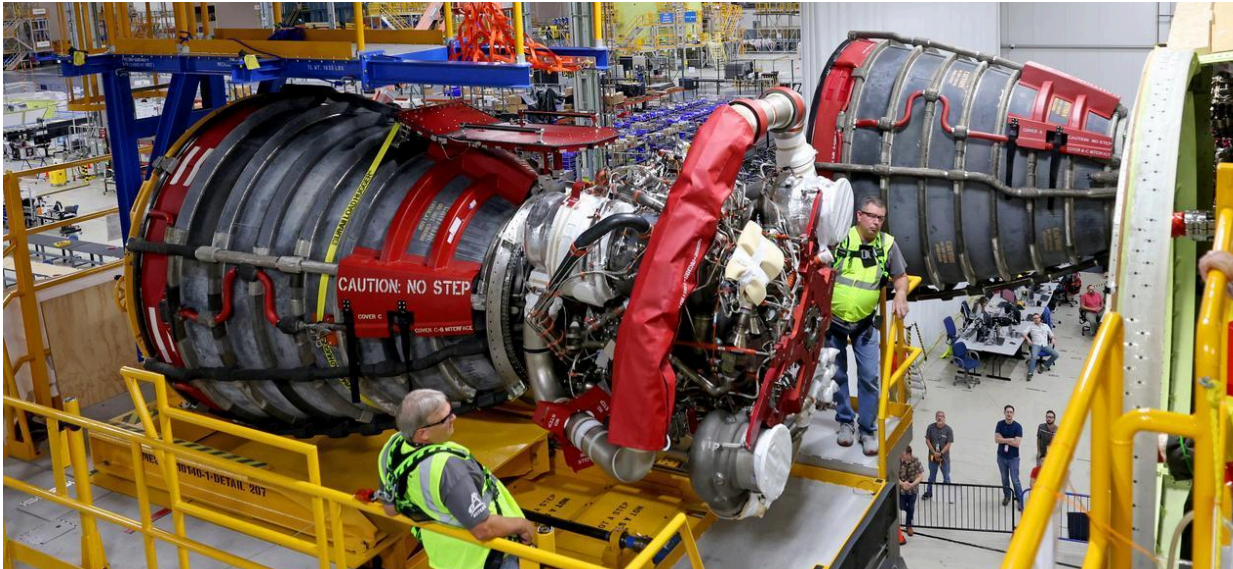
Technicians install an RS-25 engine on the Artemis II SLS core stage at NASA's Michoud Assembly Facility in New Orleans. Credit: NASA/Michael DeMocker
