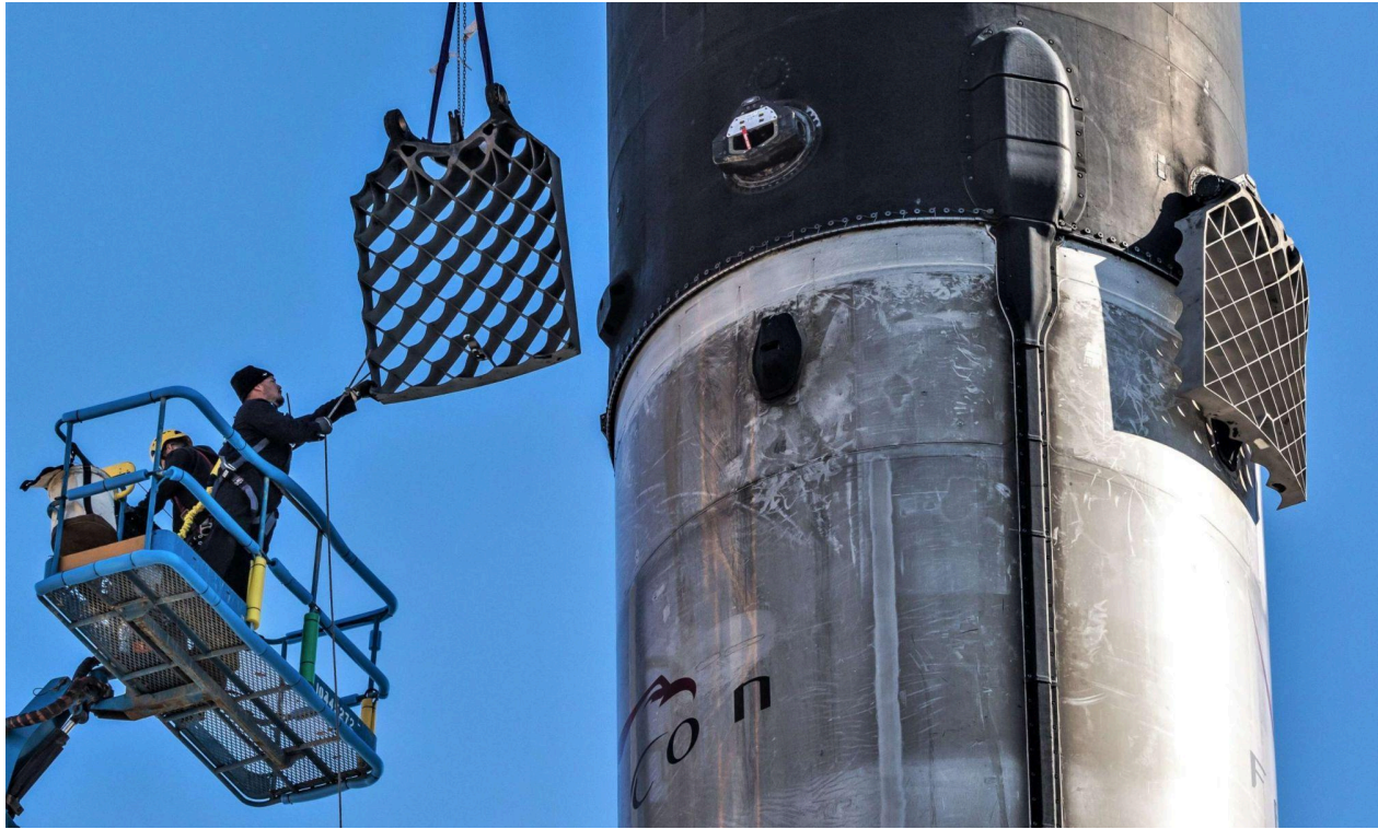
Hands on the hardware: technicians fit fins to a Falcon 9. Credit: Pauline Acalin (@pacalin)
