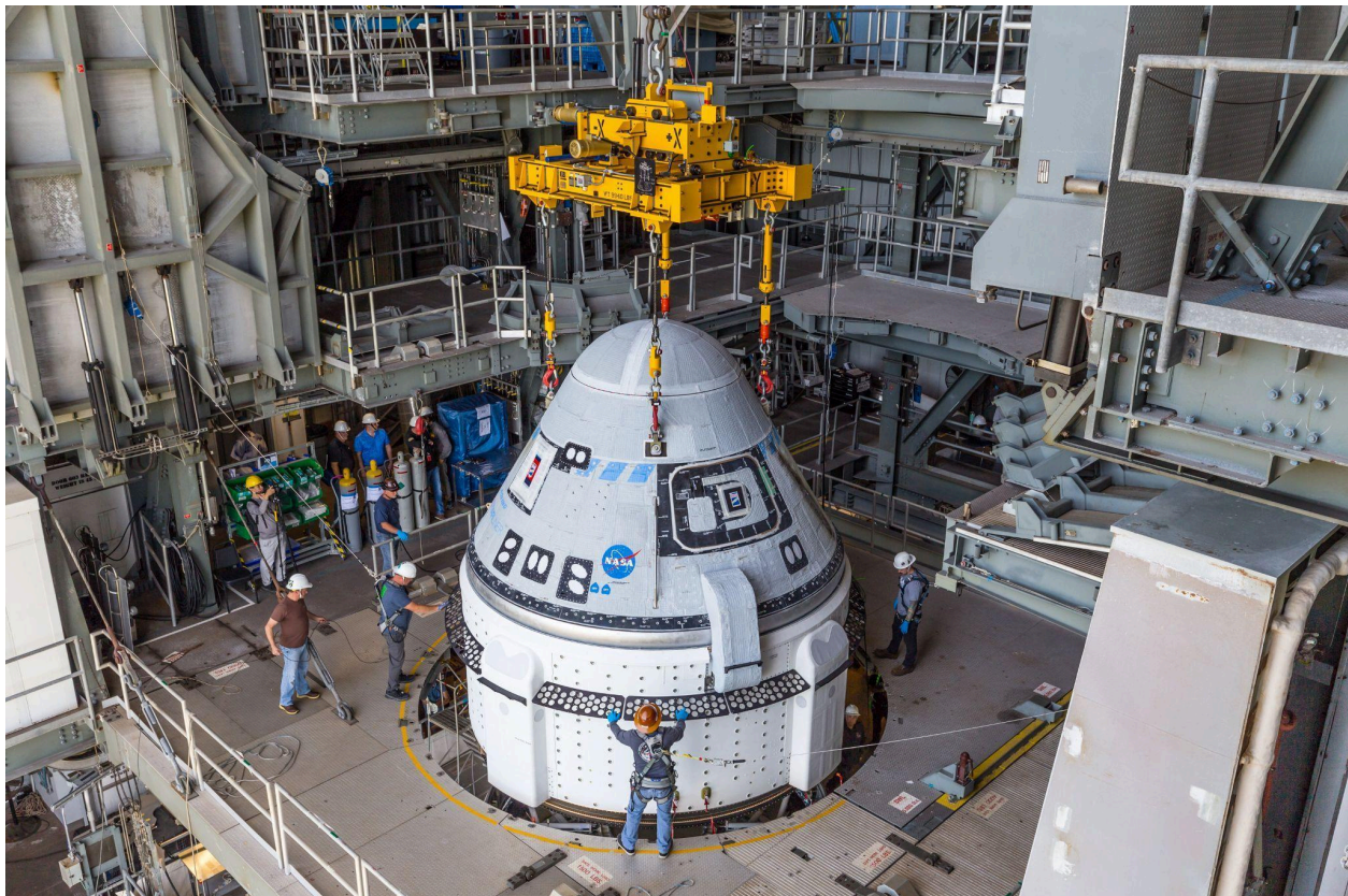
Workers guide the Boeing Starliner capsule onto its Atlas V rocket before NASA's Crew Flight Test. Credit: United Launch Alliance
