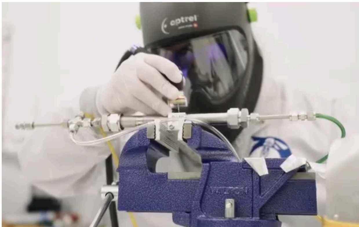
James Holster welds the feed system lines for the Blue Ghost Moon lander in the clean room at Firefly Aerospace, Cedar Park, Texas. Credit: Firefly Aerospace
