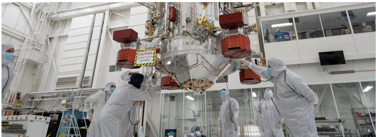
EngineerCredit: Firefly Aerospace.s lift the main body of NASA's Europa Clipper into the High Bay 1 clean room at JPL, Pasadena, California. Credit: NASA/JPL-Caltech
